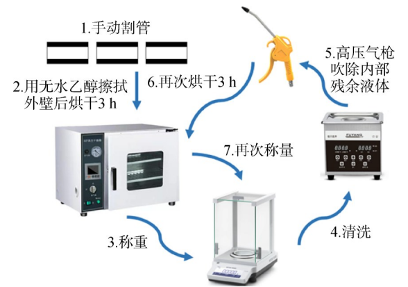
图 7 称重法流程图 Fig.7 Flow chart of weighing method
